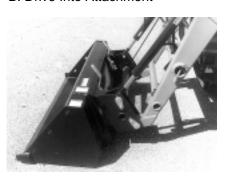
C. Raise And Roll Back Attachment D. Lower Spring-Loaded Pins
